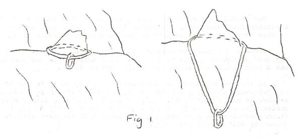
Nut slings of tape are extremely good, because the tape, being thin, can often fit into a small crack which will not admit a thick rope.
