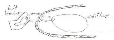
The BELAY <u>must</u> be solid and must be able to withstand a strong pull up and down. Bolts, good pitons and waist level thread belays are best.
