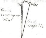
The relationship between true north, grid north and magnetic north is shown diagrammatically for the centre of the map. Magnetic value is correct for 1965. Annual change is 0003' easterly.
