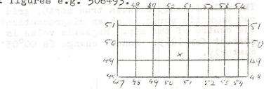
The third and sixth figures of the reference are obtained by dividing the distance between grid lines into tenths. You read the N-S grid reference first i.e. 506 is obtained from the numbers along the northern and southern boundaries of the map, and the E-W references second i.e. 493 is obtained from the numbers on the E. & W. sides of the map.
