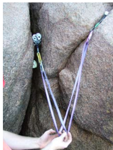
In the self-equalising or sliding-X system, twist the back strand as you pull it down into the V, then clip through the loop created by the twist and over the front strand of the sling.
