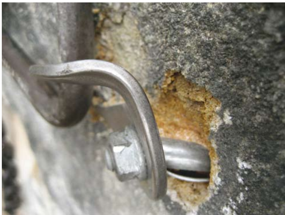
Tripod pulling a Ubolt on soft sandstone, failure at 38 kN (opposite).
